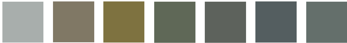
Mouse Grey RAL7005 Beige Grey RAL7006 Khaki Grey RAL7008 Green Gray RAL7009 Tarpaulin Grey RAL7010 Iron Grey RAL7011 Basalt Grey RAL7012
